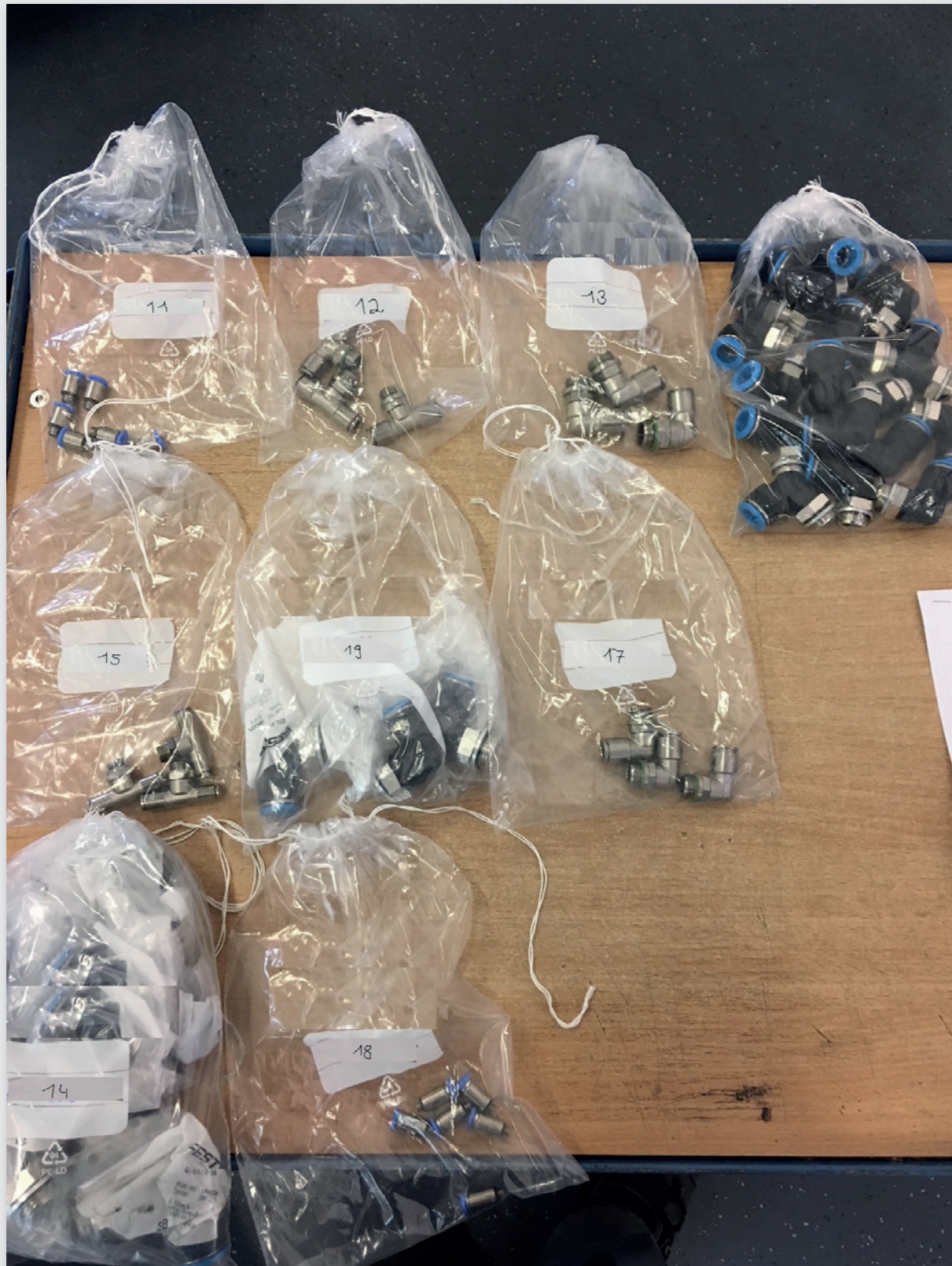
WRONG: The packaged parts are sorted and labelled with the material number of the supplier.
