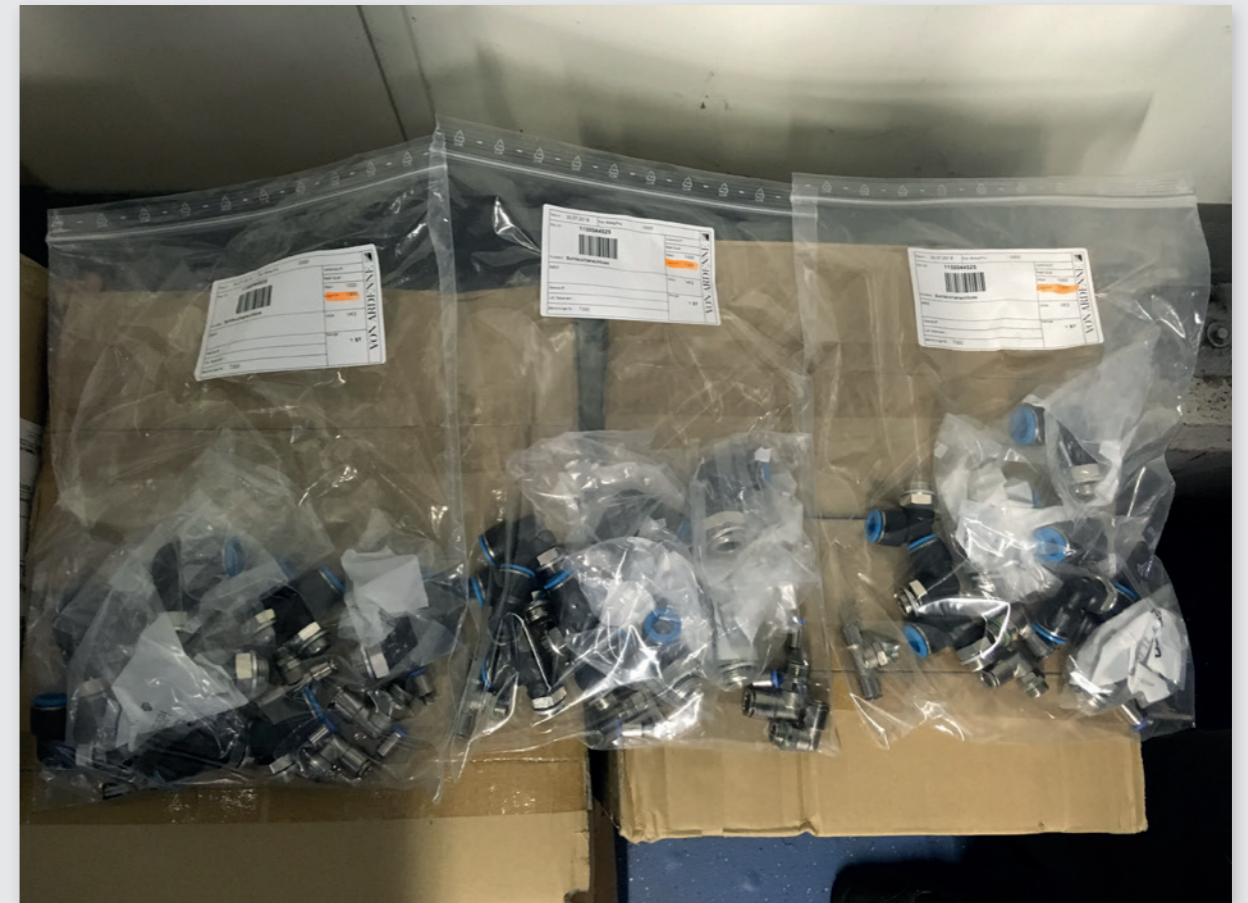
RIGHT: The parts are packaged per SET and labelled with the VON ARDENNE item number of the respective subassembly.
